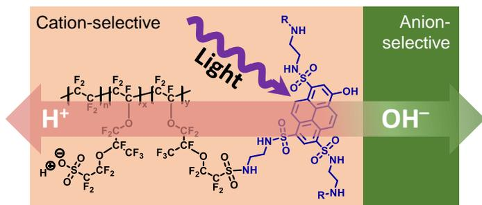
**Figure 1.** Proposed general structure and overall sensitization process for a photoacid-dye-modified bipolar
